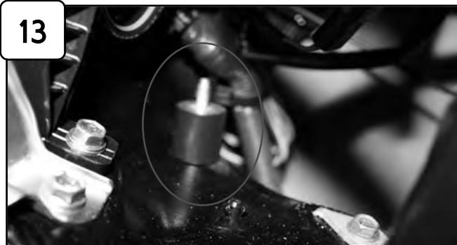
13 Install and tighten isolation mount to frame.
