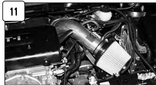
11 Install air filter and tighten using 5/16" nut driver. Tighten all clamps using 5/16" nut driver. Your short ram intake is now complete.
