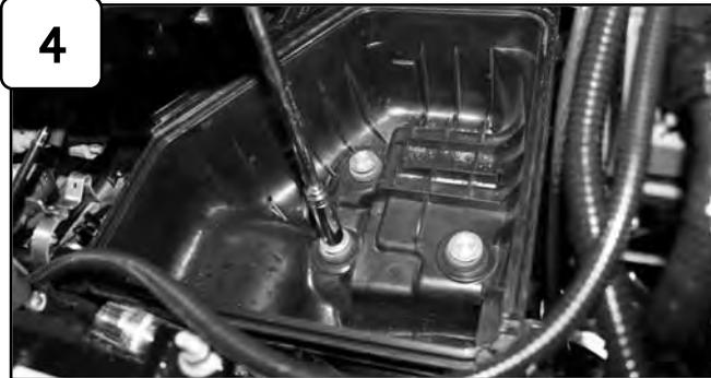
4 With 10mm socket or wrench loosen the 3 bolts holding in bottom half of air box and remove.
