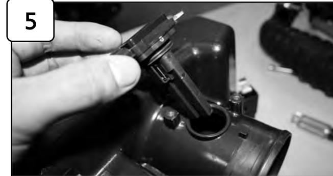
5 With phillips screwdriver loosen and remove MAF sensor.
