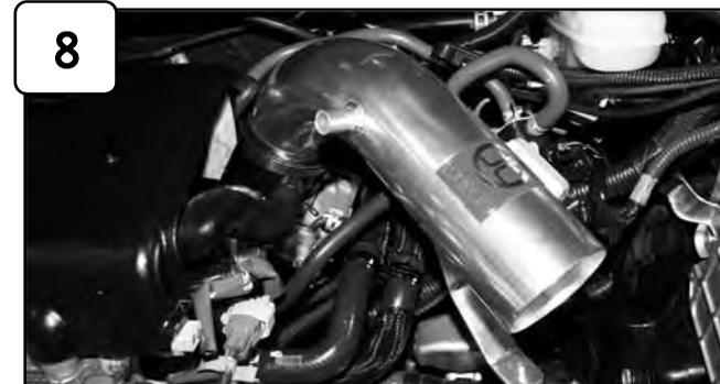
8 Install upper intake tube assembly into vehicle with provided reducer coupling and clamps. Do not tighten.
