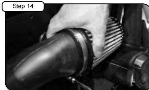
Remove front driver seat and install transmission CVT filter(18-09001) tighten using 5/16" nut driver. (CVT and mini crank case filter require no oil)
