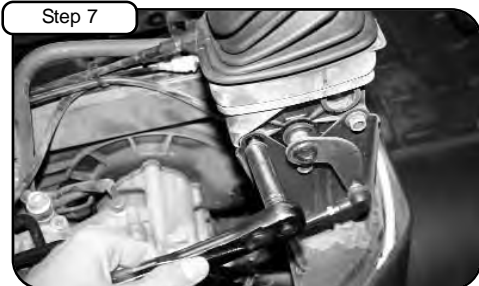
Loosen shifter bracket bolt with 12mm socket or wrench. Take bolt out and set aside for later use.
