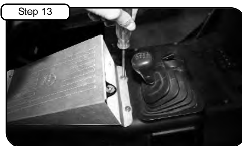
Install flat panel dry filter into cover. Tighten filter retainer bolt to cover. Tighten down aFe cover to engine housing cover using OE screws using phillips screw driver.
