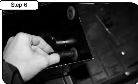
With grommets provided, place into holes in housing. Install plastic hose fitting in right side of housing.
