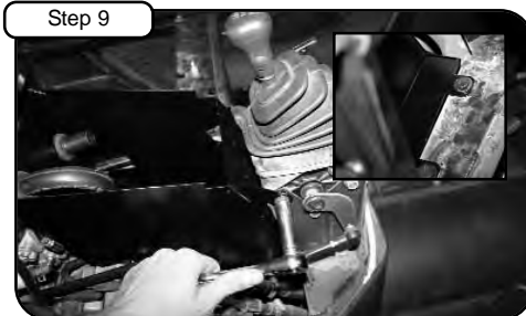
Re-tighten 12mm bolt from step 7 through housing tab and also Re-insert plastic tabs into new housing. Tighten clamps at coupler with 5/16" nut driver.
