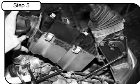
Remove the two plastic tabs holding in front of OE airbox, and save for later use. Remove complete OE airbox from Rhino.
