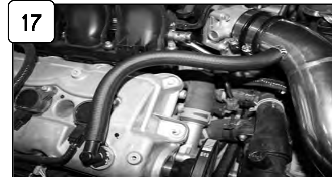
17 Install provided 5/8" hose to engine and intake tube.
