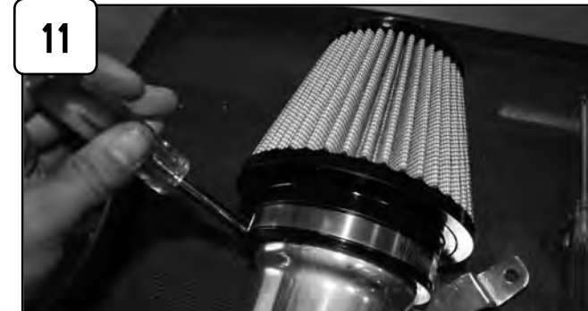
11 Attach air filter and tighten using 5/16" nut driver.
