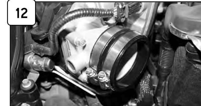
12 Attach coupling to throttle body using provided clamps. Do not tighten.
