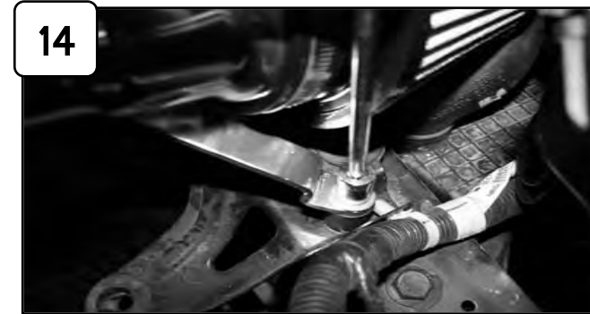
14 Using provided flat washer and nut, secure tab using 13mm socket or wrench.
