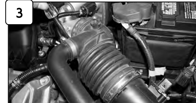
With 5/16" nut driver loosen clamp on throttle body. Disconnect MAF sensor harness.
