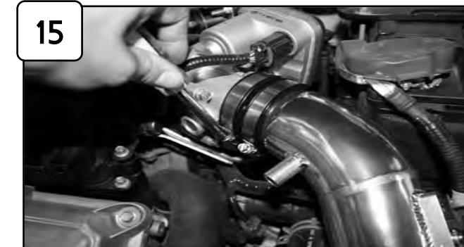
15 Tighten all clamps using 5/16" nut driver.
