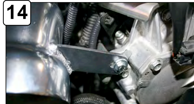
14 Secure tab to engine and tighten using provided screw and flat washer.
