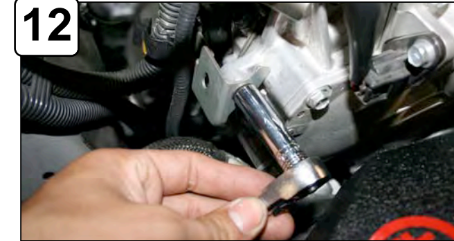
12 Loosen bolt on engine securing harness bracket.
