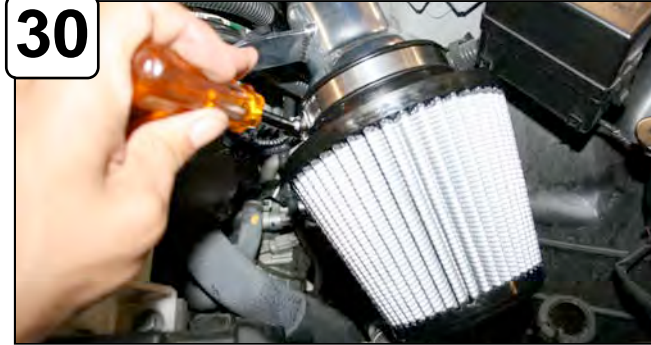
Tighten all clamps using 5/16" nut driver. Install air filter and tighten using 5/16" nut driver.
