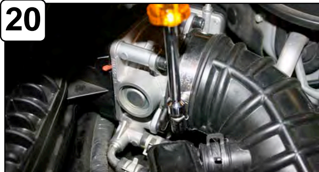
Disconnect MAF sensor harness. Loosen clamps using 5/16" nut driver.
