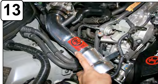
13 First re-connect MAF sensor harness. Install into vehicle and position tube. Do not tighten clamps.
