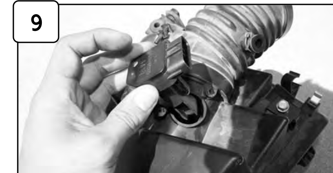
With phillips screwdriver, loosen and remove MAF sensor from stock air box.
