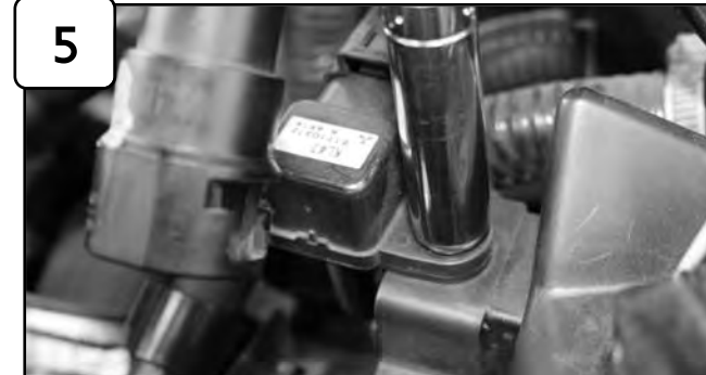
With 10mm wrench loosen VSV valve on air box, disconnect and remove. Save for later install (See step 11).
