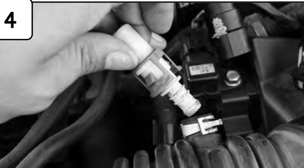
Disconnect Crank case line and remove plastic fitting. Save for later install (See step 11).
