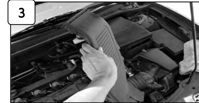
Remove plastic battery ram air.
