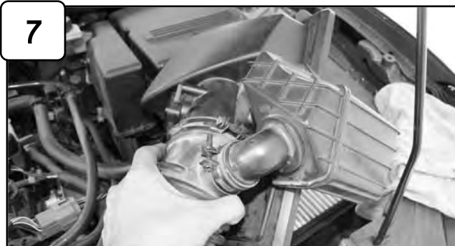
Lift and remove upper half of air box.
