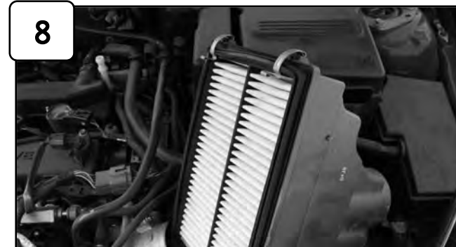
Remove bottom half of air box.
