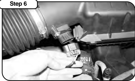
Unplug electrical harness from MAF sensor, location shown in figure B on step 5.
