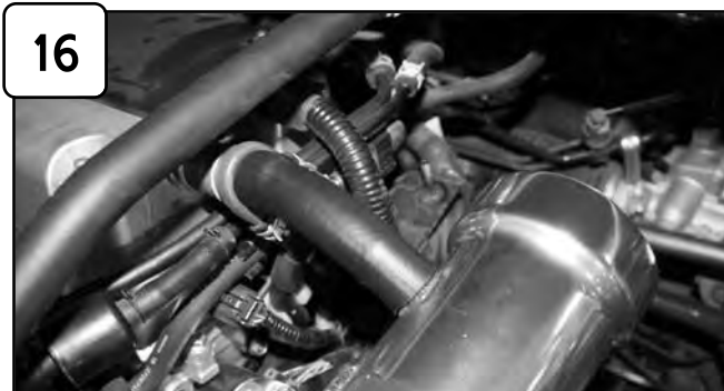
16 With provided 5/8" hose connect to engine and tube.
