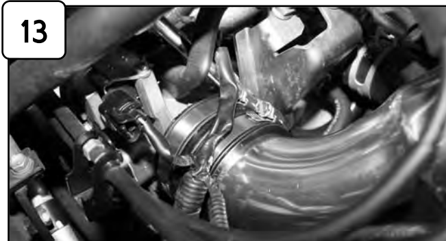
13 Tighten clamps using 5/16" nut driver.
