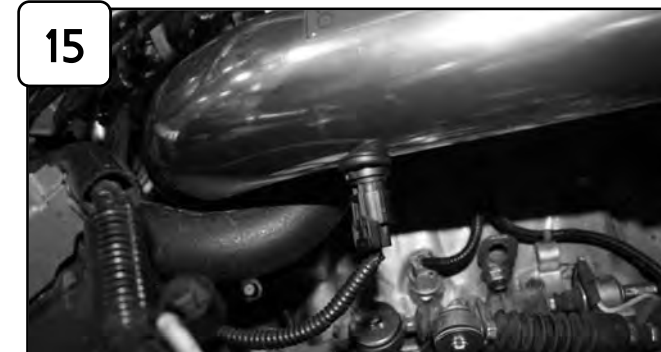
15 Install temp sensor to grommet on tube and connect sensor harness.
