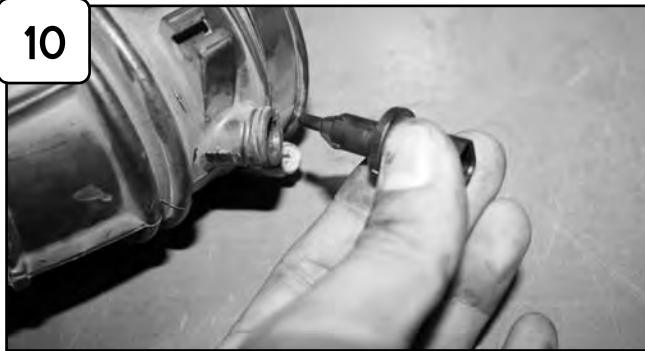
10 Remove temp sensor from stock intake tube.
