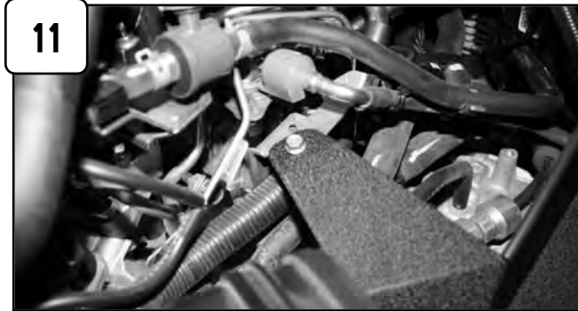
Install housing into vehicle and position. Re-secure tab on housing with bolt from step 10.
