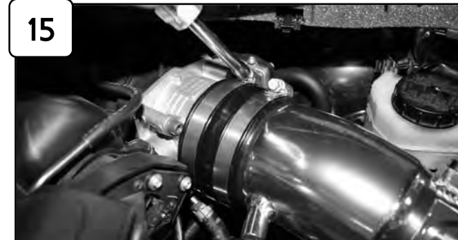
Tighten all clamps using 5/16" nut driver.
