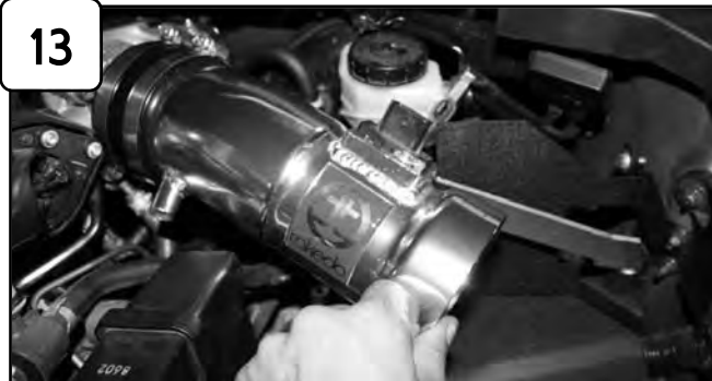
Install intake tube assembly and position tab to isolation mount. Do not tighten.
