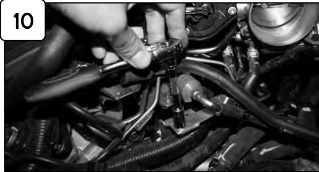
With 10mm socket or wrench loosen bolt on engine.
