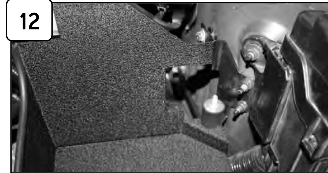
Secure housing with isolation mount. Secure small tab using M6 screw, wavy washer and nut. Tighten all screws and bolts using 10mm socket or wrench.
