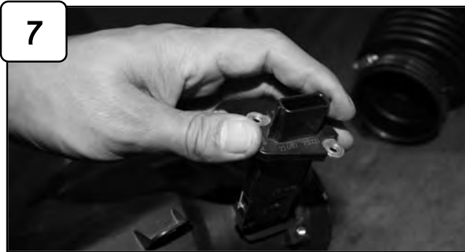
Remove MAF sensor using phillips screwdriver.
