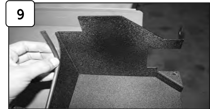
Attach rubber trim to housing.
