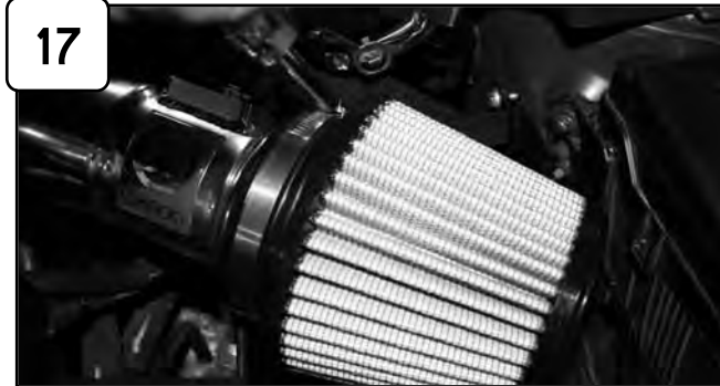
Install air filter and tighten using 5/16" nut driver. Re-connect battery terminals.
