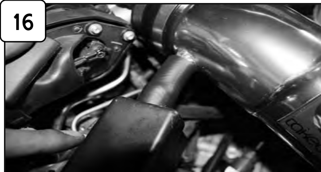
Attach 5/8" hose from the crank case port on the intake to the stock plastic vacuum port. Re-connect MAF sensor harness.
