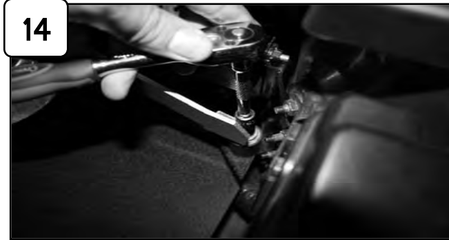
Tighten intake bracket using provided flat washer, wavy washer and nut.
