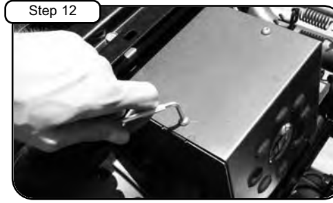
Step 12 Secure cover to housing using M6 allen head bolts.
