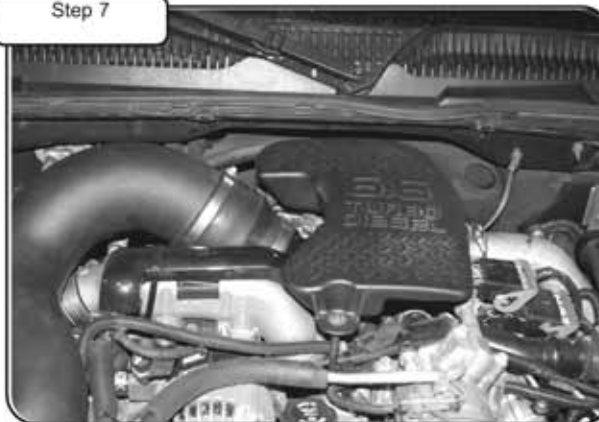
Re-attach resonator plenum on aFe turbo inlet tube. Tighten clamp with flathead screw driver or 1/4" socket driver. Re-install mounting screw with T30 Torx driver. Your installation is now complete. Thank you for choosing aFepower!
