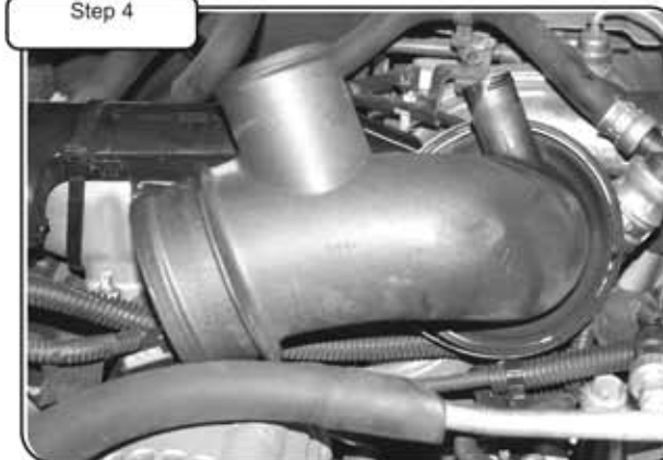
Loosen turbo inlet tube flange clamp with 5/16" socket driver. Remove stock turbo inlet tube from truck.
