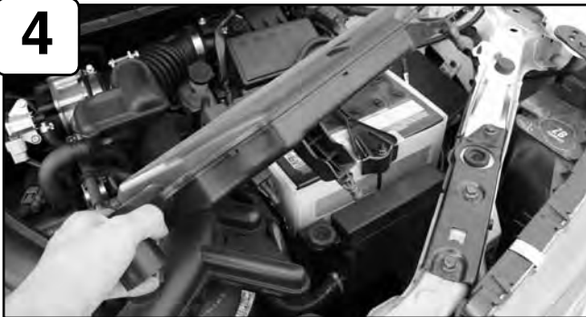
Remove stock resonance chamber.
