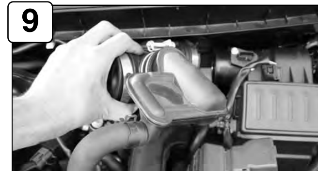
Remove the stock intake tube.
