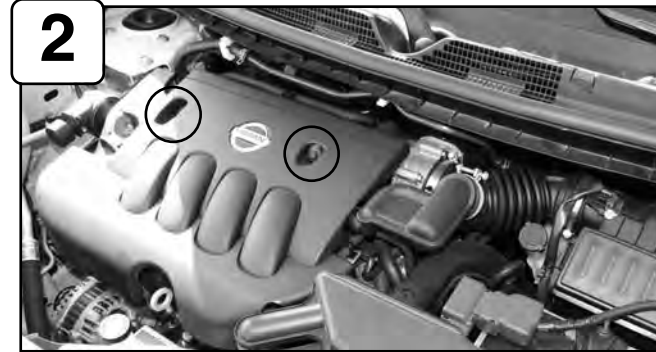
Complete Stock intake. Remove two screws holding the engine cover into place.
