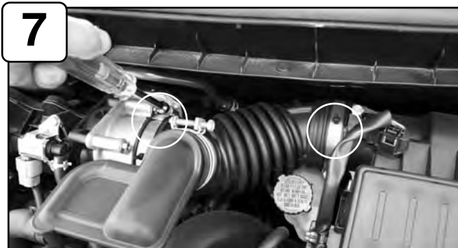
Using a 5/16" nut driver, loosen both intake tube clamps circled.
