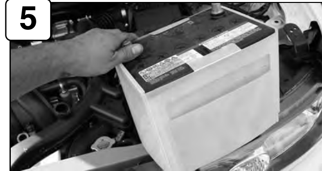
Disconnect battery terminals and remove battery.
