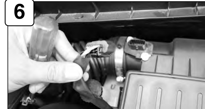
Disconnect the MAS sensor.
