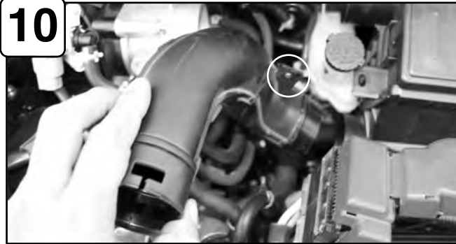
10 Remove wiring harness attached to stock ram air duct, and pull out the stock ram air duct from the vehicle.
