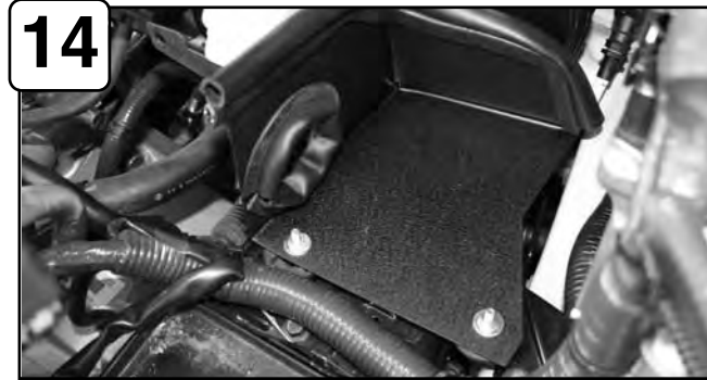
14 Place housing into the vehicle reusing the stock mounting locations.
