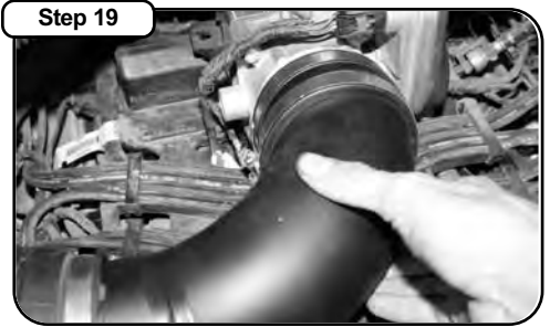
Insert intake tube to factory accordion tube.
