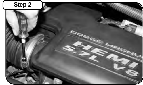
Loosen clamp on inlet tube to intake plenum
