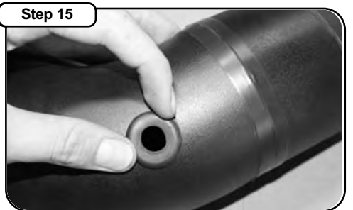
Insert supplied grommet into hole on intake tube
