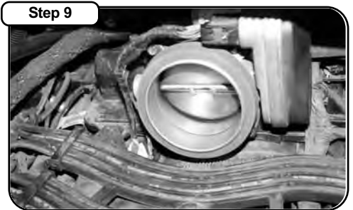
Remove rubber seal from throttle body
