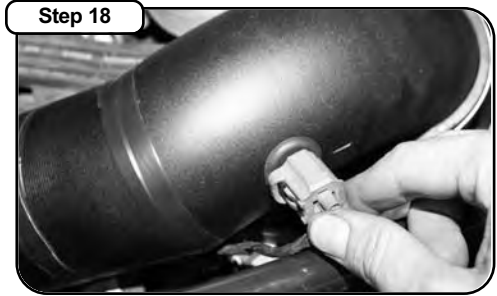
Re-connect electrical connector to temp sensor and throttle body
