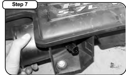
View of intake plenum removed from vehicle
