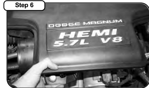
Remove intake plenum from vehicle
