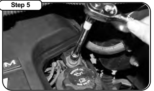
Remove intake plenum mounting bolt
