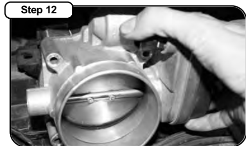
Remove throttle body from vehicle
