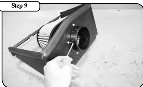
Secure the air filter adapter to the housing using the (5) M6 allen bolts provided. Then place filter onto filter adapter and tighten the clamp.
