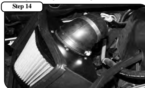
Place the elbow coupling onto the adapter but do not tighten clamp until later.
