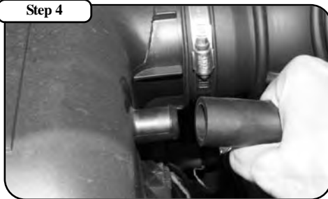
Unplug the crank case breather tube.
