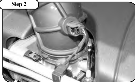
Loosen the clamp at the throttle body.
