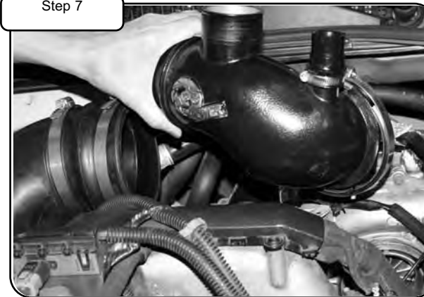
Install aFe turbo inlet tube. Ensure flange clamp fits correctly on aFe turbo inlet tube and turbo compressor housing. Do not tighten flange clamp.
