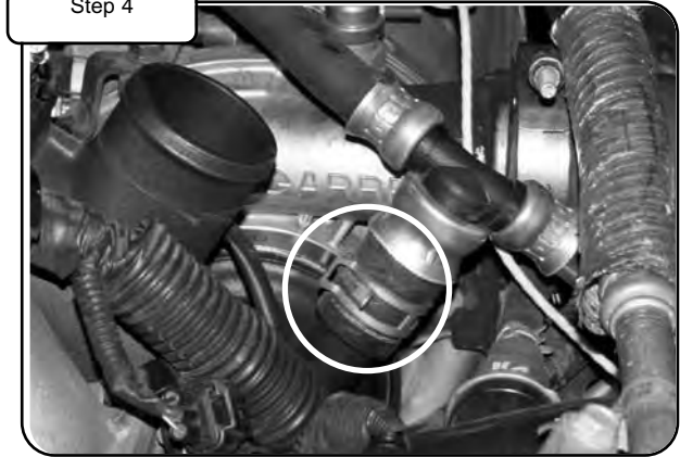
Open clamp on CCV hose coupling with pliers and remove hose coupling from the stock turbo inlet tube.
