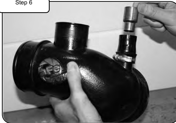
Install supplied CCV coupling adapter and mini hose clamp on aFe turbo inlet tube. Tighten with flat tip screwdriver or 1/4" socket driver. Insert supplied copper coupling into CCV coupling adapter as shown.
