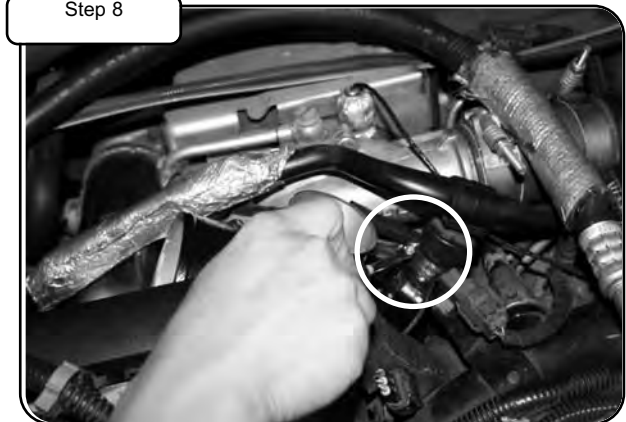
Re-attach CCV hose coupling on aFe turbo inlet tube using supplied mini hose clamp. Tighten with flat tip screwdriver or 1/4" socket driver. Re-attach CCV hose end on passenger side of truck.
