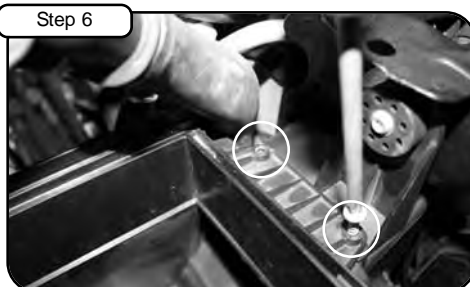
Loosen the 2 screws holding in bottom part of air box using phillips screwdriver. Note: Bottom part of air box consists of two separate pieces.
