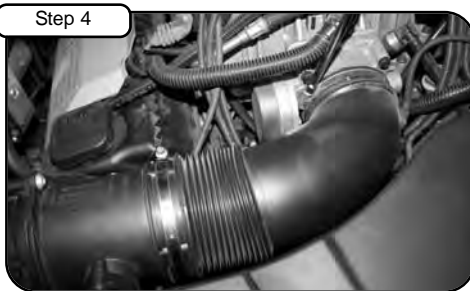
Loosen all clamps at Throttle Body and MAF sensor with 8mm nut driver. Disconnect vacuum line from tube.
