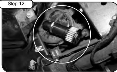
With 18-01004 filter, attach to plastic fitting and tighten using 8mm nut driver. Install to smog pump.
