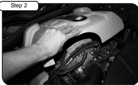
Remove engine cover using 4mm allen key.
