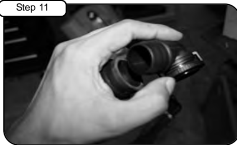
With pliers, cut existing clamp and remove plastic elbow fitting.
