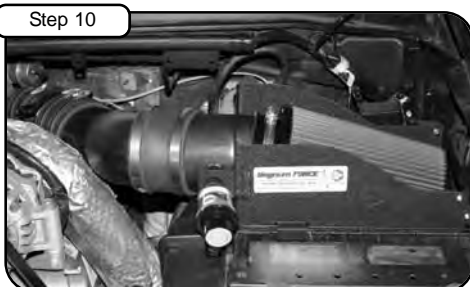
Step 10 Your aFe intake installation is now complete. Make sure all clamps are tight and that all electrical components are secure. Check and tighten connections after a few hours of operation. Thank you for choosing aFepower!
