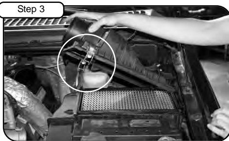
Step 3 Loosen the air box lid clamps and remove air box lid and OEM air filter.
