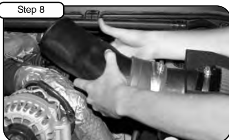
Step 8 Slide coupler and clamps on tube. Position assembly into the intake kit.
