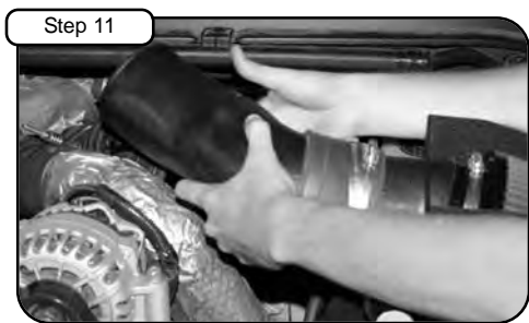
Slide coupler and clamps on tube. Position assembly into the intake kit.
