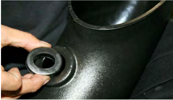
10- Install supplied grommet into aFe's intake tube.
