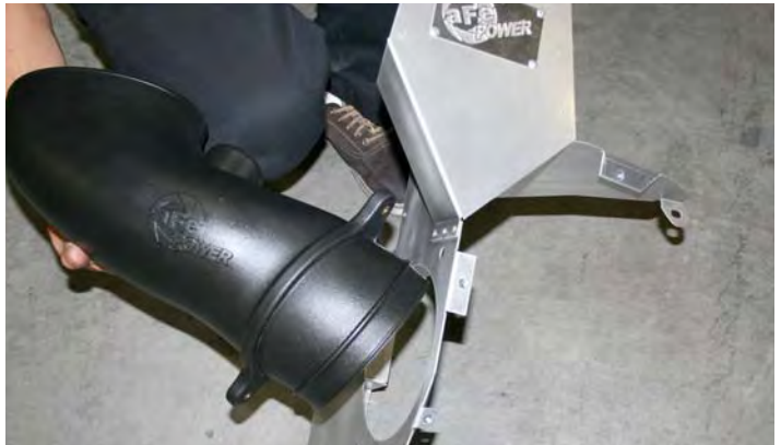
8- install aFe's intake tube into the housing.
