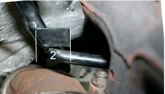
4 – View of the cut bracket.
