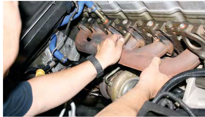
7 – Remove the stock manifold bolts using 13mm deep socket and save them for later install. After removing the stock manifold, clean the head and turbo surface to improve the seal.
