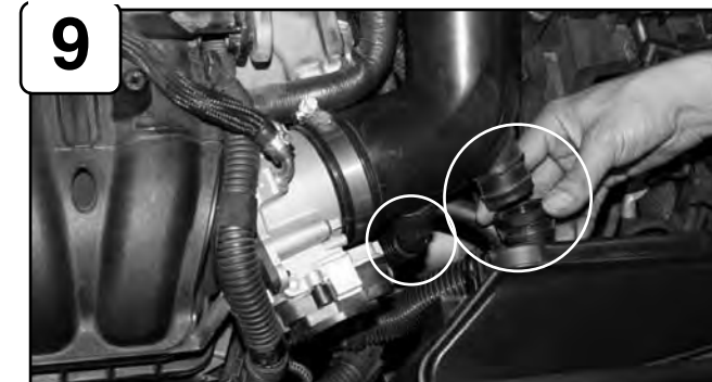
Disconnect both smog pump adapters.
