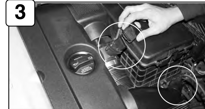
Disconnect MAF sensor and crank case line.
