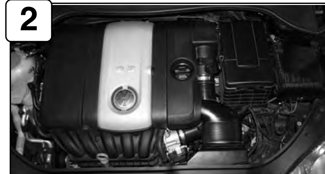
Complete Stock intake. Please disconnect battery terminals before installation. Be sure to have your radio security code (if applicable) in order to access your previous settings.
