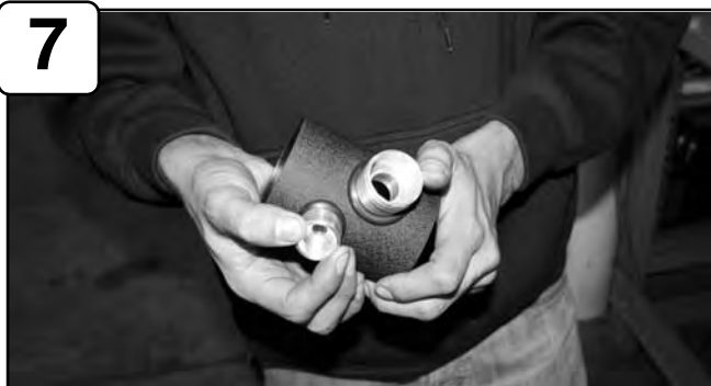
Install both grommets onto your takeda intake tube then firmly press in both smog pump adapters.
