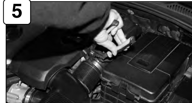
Using pliers, squeeze the pressure clamp open and pull the factory tube off the mas sensor tube.
