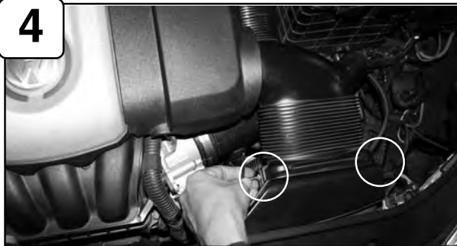
With an allen wrench, Unscrew both screws holding the ram air duct into place.
