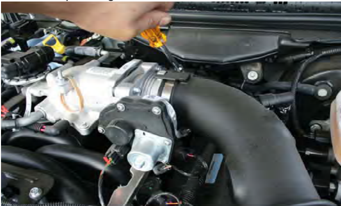
3- Loosen the clamp at the throttle body
