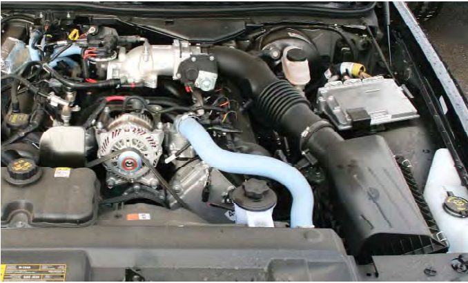
1- View of stock intake system.
