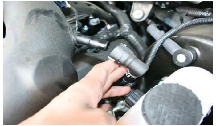
5- Disconnect the crank case line from the intake tube.
