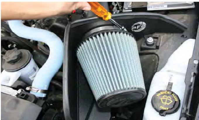
19- Connect your aFe air filter onto your housings adapter.
