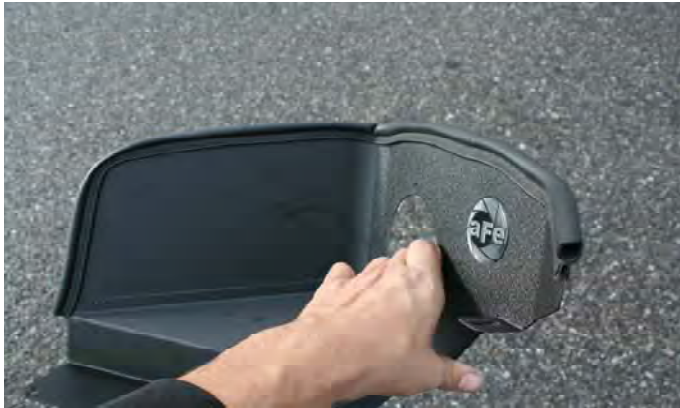
9- Firmly place the supplied seal trim on the housings top edge.
