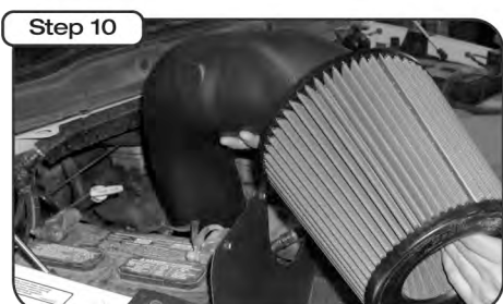
Install new tube into vehicle, slide coupler onto turbo inlet, fasten clamp assembly securely.
