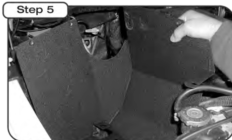
Install new intake housing into vehicle.
