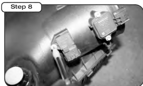
(6.7L remove and install temp sensor, see step 7) 6.7L, remove MAF sensor and install to new tube with screws and gasket (Make sure gasket is between sensor and tube) Install grommet only to tube. The 6.7L will not use small phillips screws.
