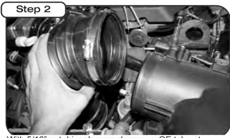
With 5/16" nut driver loosen clamps on OE tube at turbo/air box and remove. (6.7L remove crank case line with pliers and save OE plastic fitting for later install)
