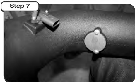
With T-20 torx bit remove temp sensor and (with gasket and screws provided) install into new tube. (5.9L place MAF cover with gasket and tighten using short phillips screws provided. Install plug into the hole in tube for crank case line)
