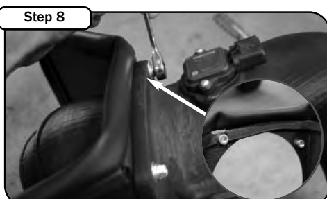
Step 8 Install trim seal to housing, make sure cutout is at pem-nut on housing. Install tube to outside of housing. Tighten using hex screws, split and flat washers provided with 3/8" socket or wrench.
