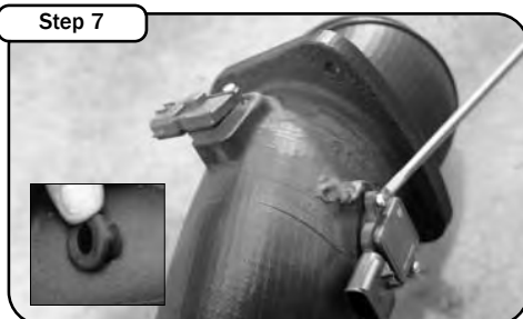
Step 7 Insert MAF sensor and temp sensor into new tube with gaskets and #8-32 screws provided. Tighten using flathead screwdriver. Install filter minder grommet in hole provided and install filter minder.
