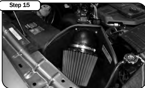
Step 15 Place the included CARB EO Sticker on or near the intake system on a smooth, clean surface. E.O. identification label is required in passing the Smog Check Inspection. Your installation is now complete. Check all clamps and connections. Periodically check all clamps and hoses. Thank you for choosing aFe!
