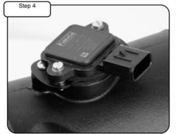
install MAF sensor using Flat head screws. Your installation is now complete.
