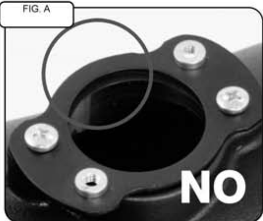
INCORRECT: If there is an overlay it will not allow the MAF sensor to be installed correctly. Turn 180° and it will correct this issue.
