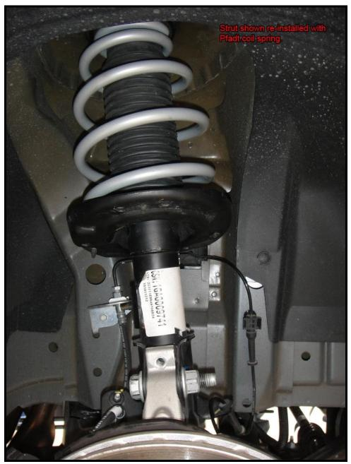
Figure 8 - Front Strut with Pfadt Drop Spring
