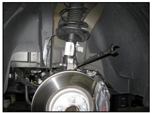
Figure 4 - Removing Spindle to Strut Bolts
