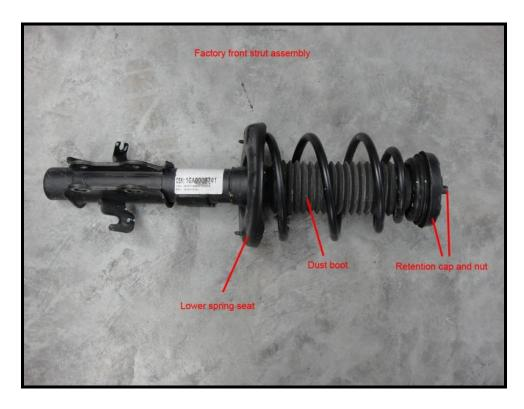
Figure 5 - Front Strut Removed from Vehicle
