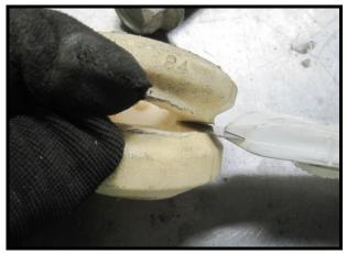
Figure 7- Trimming Front Bump Stop
