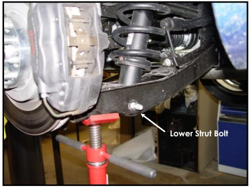
Figure 10 - Lower Strut Bolt
