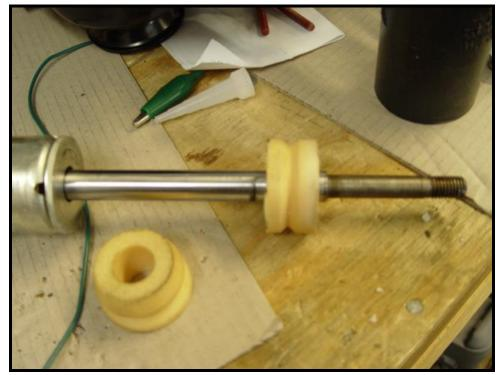
Figure 15 - Strut with cut Bump Stop
