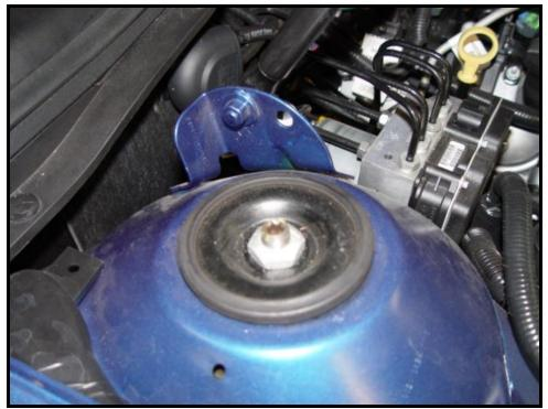
Figure 2 - Upper Nut and Strut Retaining Plate
