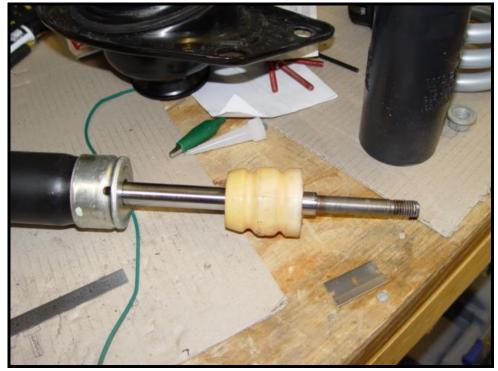
Figure 14 - Strut with un-cut Bump Stop
