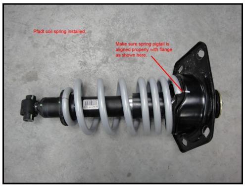
Figure 16 - Assembled Rear Strut
