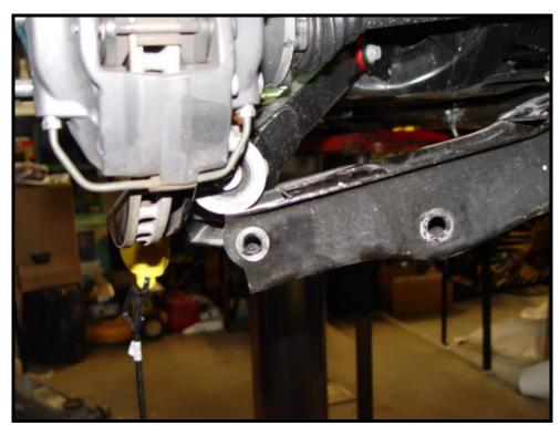
Figure 11 - Lower Control Arm to Spindle Bolt Location
