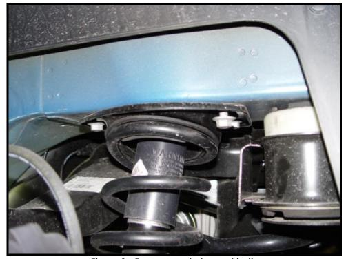
Figure 9 - Four upper strut mount bolts
