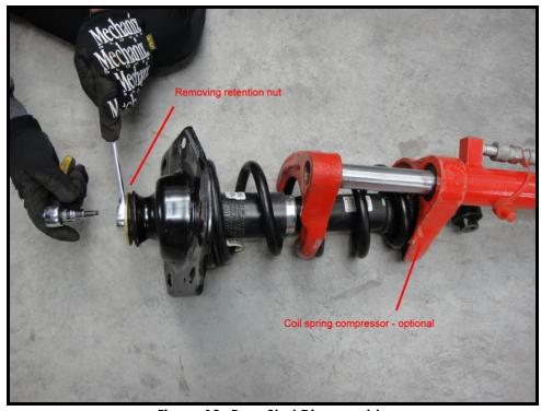
Figure 13- Rear Strut Disassembly
