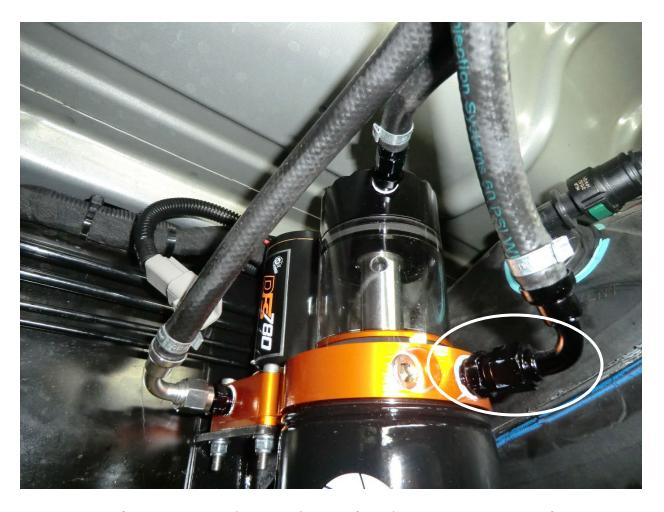
36. Install the fuel outlet hose (black  $90^{\circ}$  -6 AN fitting) onto the male -6 AN fitting on the fuel outlet port of the fuel manifold assembly.
