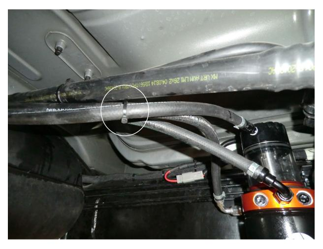
38. Route the hoses as shown and secure with the supplied nylon cable ties.
