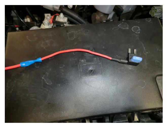
48. Attach the power wire from the relay harness to the supplied add a harness fuse adapter.
