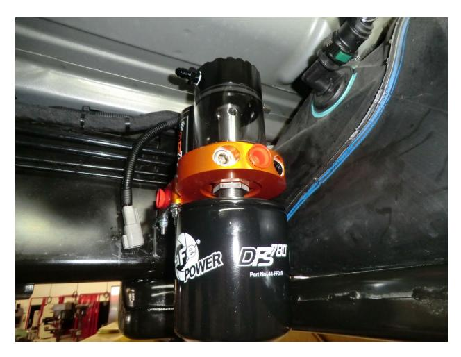
11. Using a light oil, lube the gasket on the supplied fuel filter and install on the fuel manifold assembly. Thread the supplied water separator bowl onto the fuel filter.
