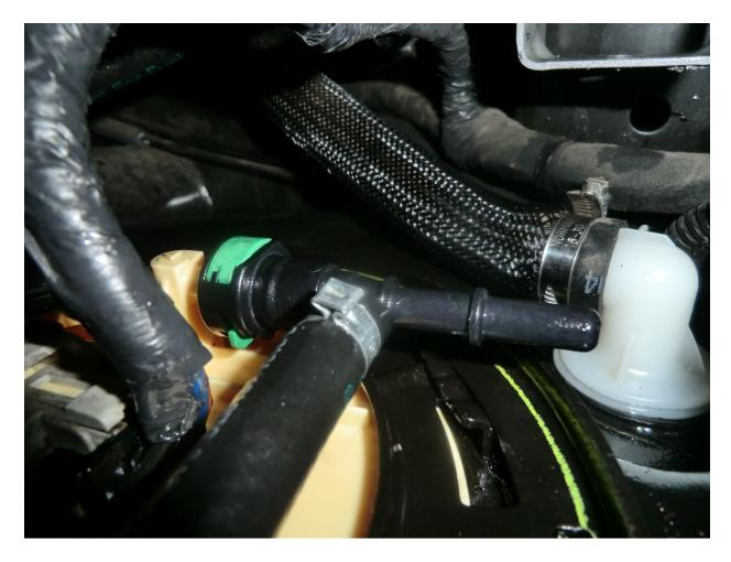
29. Install the female side of the "T" quick disconnect fitting on the supplied fuel return hose (shown below) onto the male fuel return connection on the top of the fuel sender assembly.
