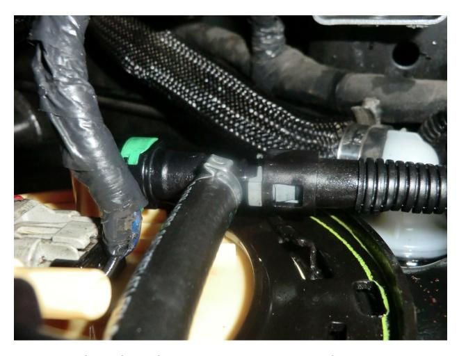
31. Install the factory female fuel return line onto the male side of the "T" quick disconnect fitting on the fuel return hose (shown below).
