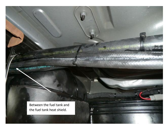
34. Route the new hoses along the DEF fill tube, between the fuel tank and the fuel tank heat shield. Secure with the supplied nylon cable ties (as shown above).
