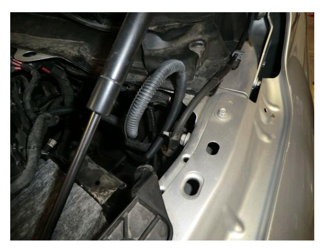
42. Run the other end of the power harness along the inside of the frame into the engine compartment.
