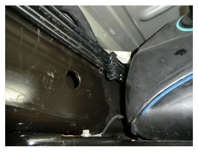
2. Gently pull the hard lines off the frame rail. Be careful not to bend or kink the hard lines.
