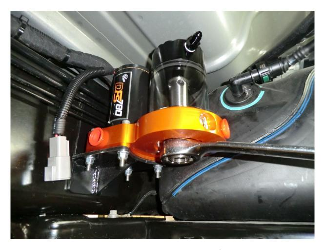
10. Turn the sight glass to the desired angle and using a 1-1/4" wrench, tighten the center nut under the fuel manifold assembly.
