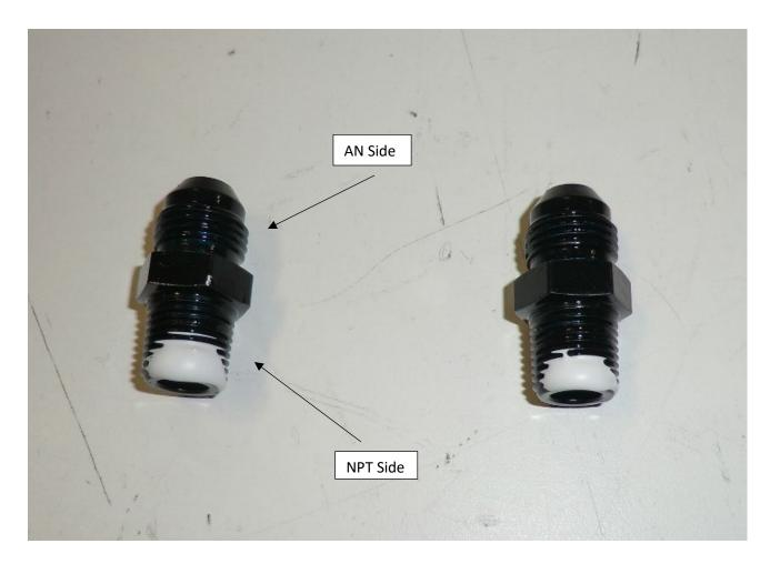
12. Apply Teflon tape with PTFE (or Teflon paste with PTFE) to the supplied fittings.
