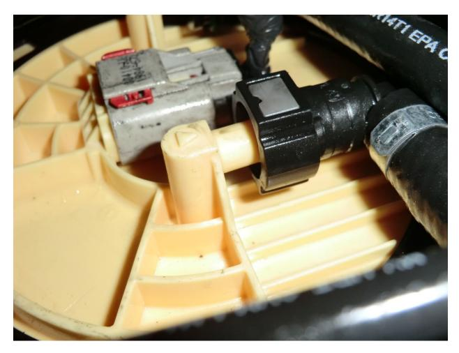
32. Install the  $90^{\circ}$  female quick disconnect fitting on the supplied fuel inlet hose (silver  $90^{\circ}$  -6 AN fitting as shown below) onto the male fuel feed connection on the top of the fuel sender assembly.
