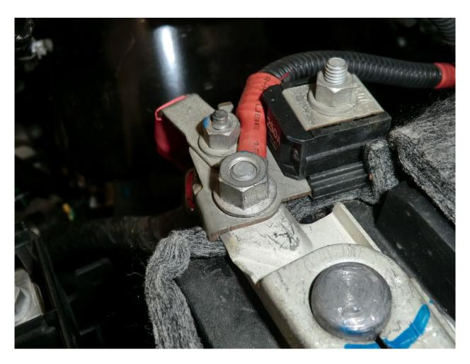
43. Connect the red wire ring terminal on the power harness to the positive side of the battery.
