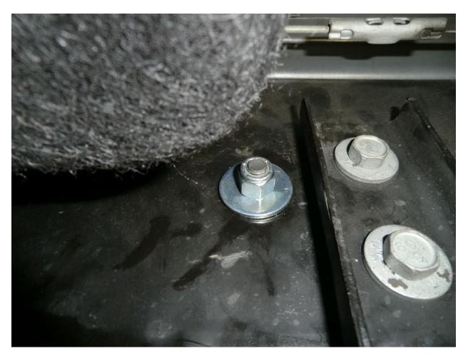
7. Using the supplied 3/8 locknut and 3/8" washer, tighten the bracket on to the frame rail.
