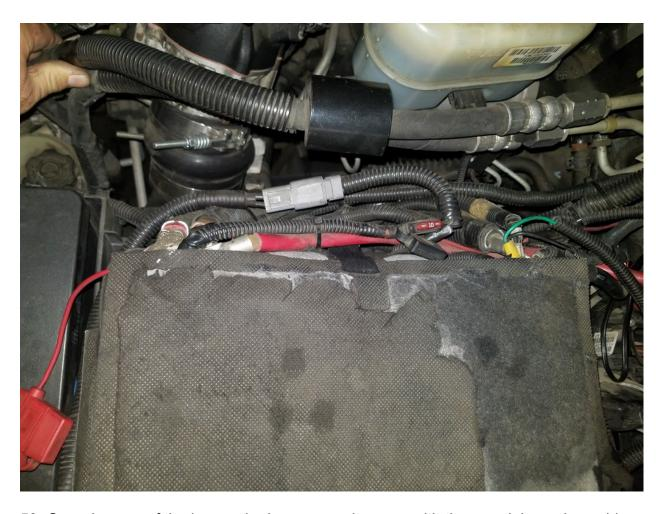
53. Organize any of the loose wire harness and secure with the remaining nylon cable ties.
