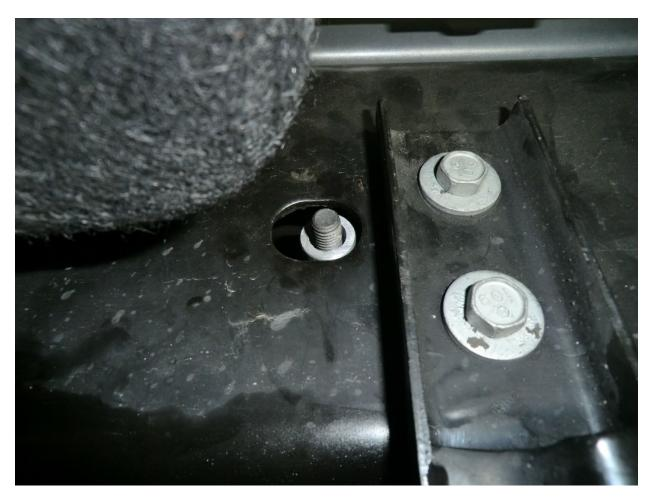
6. Install the supplied aluminum spacer onto the 3/8"-16 x 3.50" bolt.
