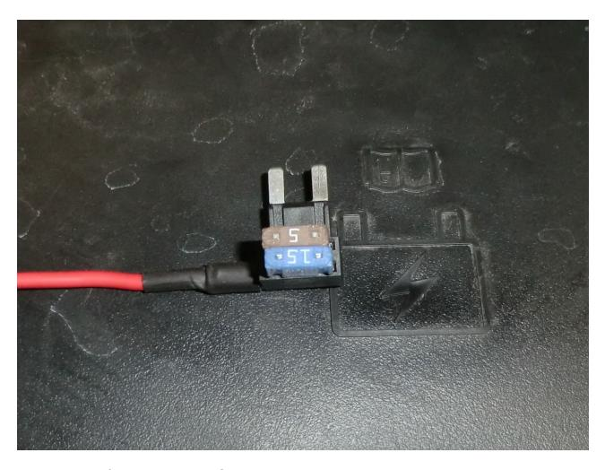
50. Install the fuse removed on Step 49 and insert it into the open location on the supplied add a harness fuse adapter (not in line with the wire).
