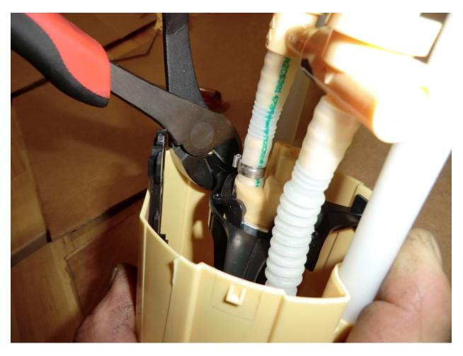
20. Carefully cut the three supports holding the factory fuel pump.
