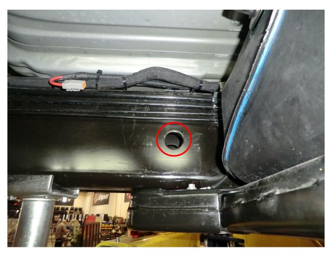
1. Locate the hole in the driver's side frame rail behind the DEF tank and in front of the fuel tank.
