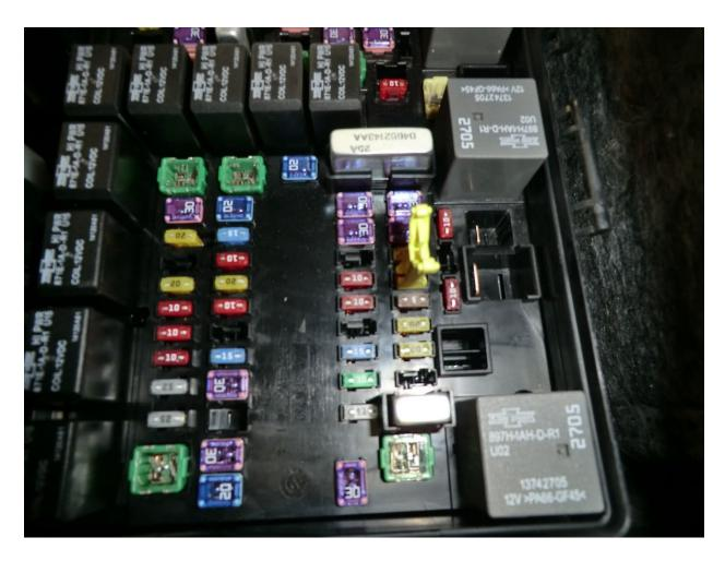
49. Find a 12-volt source inside the fuse box that only comes on with the key in the "run" position. Once a 12-volt source is located, pull the fuse from the fuse box.
