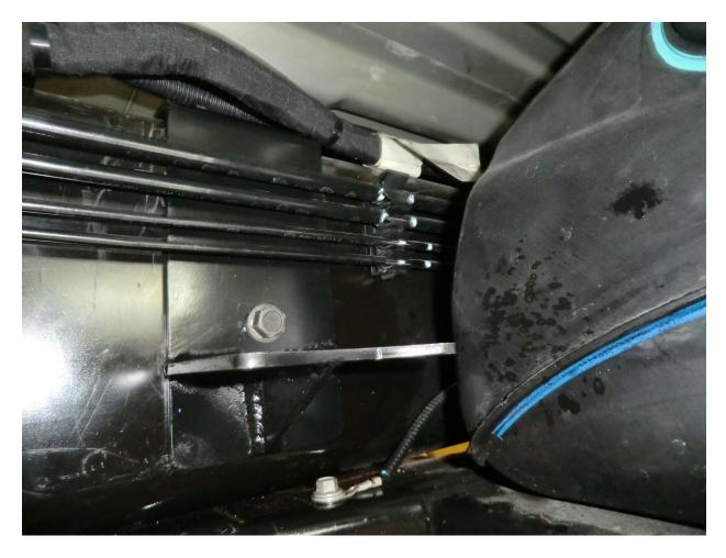
8. Re-install the hard lines onto the frame rail.
