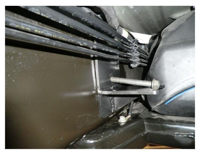
5. Install the supplied 3/8"-16 x 3.50" bolt through the carbon steel frame bracket and the frame rail.
