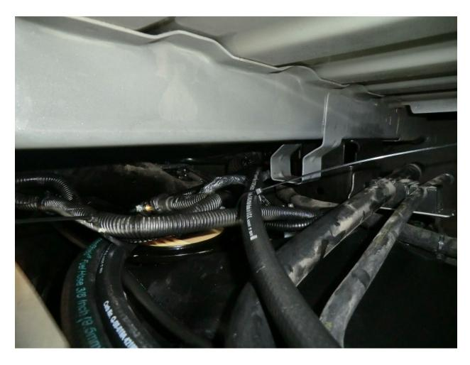
33. Route the new hoses as shown and secure with the supplied nylon cable ties.
