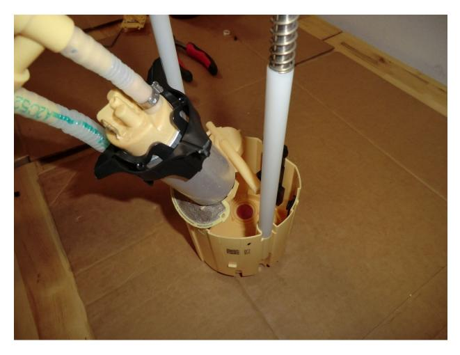
21. Remove the factory fuel pump, suction line and return line from the fuel sender assembly.
