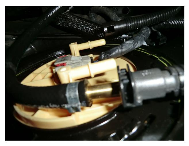
28. Install the straight male quick disconnect fitting on the supplied fuel outlet hose (black  $90^{\circ}$  -6 AN fitting - shown below) into the female side of the stock fuel feed line.
