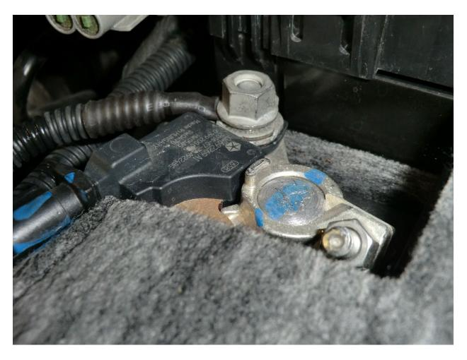
44. Connect the black wire ring terminal on the power harness to the negative side of the battery.
