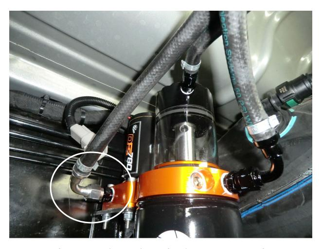
35. Install the fuel inlet hose (silver  $90^{\circ}$  -6 AN fitting) onto the male -6 AN fitting on the fuel inlet port of the fuel manifold assembly.
