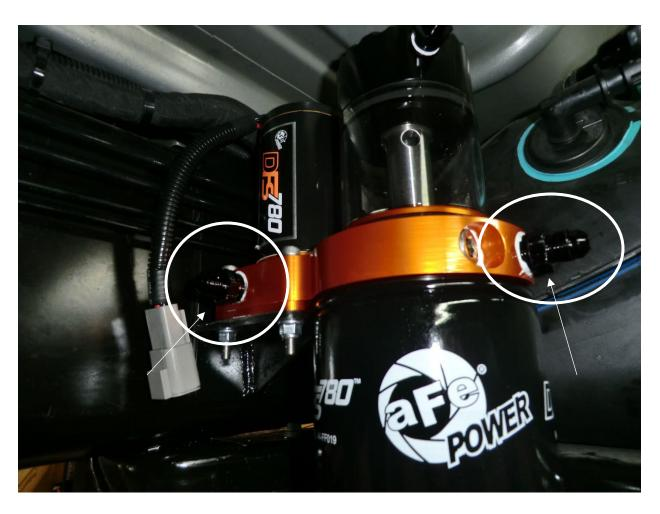
13. Install the 3/8" NPT to -6 AN fittings into the fuel manifold assembly (as shown above).
