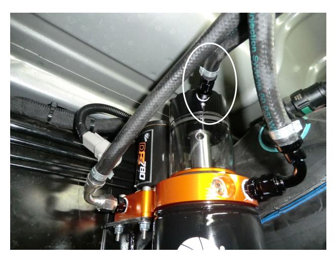
37. Install the fuel return hose (-4 AN fitting) onto the male -4 AN fitting on the top of the sight glass cover.
