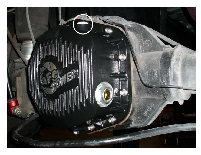
19. Apply Teflon tape/pipe sealant and install the supplied 3/4" NPT plug into the top of the cover.
