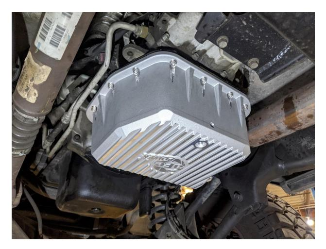
Hold the transmission pan up into position, aligning the screw holes. Install four (4) 5/16"-18 socket head screws and 5/16" flat washers into each of the corners to hold the pan into position.
