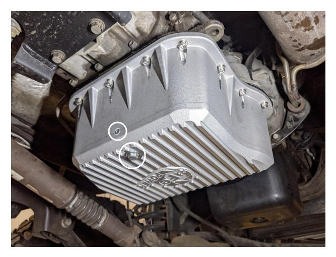
19. Install the supplied M12x1.25 magnetic drain plug and crush washer (secure about ½ turn past finger tight).
