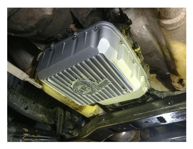
15. Hold the transmission pan up into position, aligning the screw holes. Install four (4) M6x1.0x20 socket head screws and M6 washers into each of the corners to hold the pan into place.
