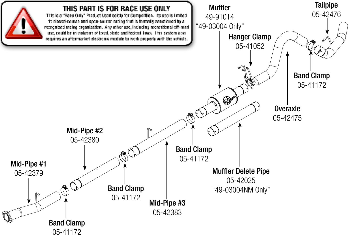
**Step 1: (Read Instructions prior to installation)** Remove the stock exhaust from the rear of the truck working your way forward. Take caution not to damage the factory isolation mounts as they will be reused. Disconnect sensors at the connections. Take caution as not to damage any sensors. **It is recommended to not fully tighten the clamps until the entire system has been installed.**
