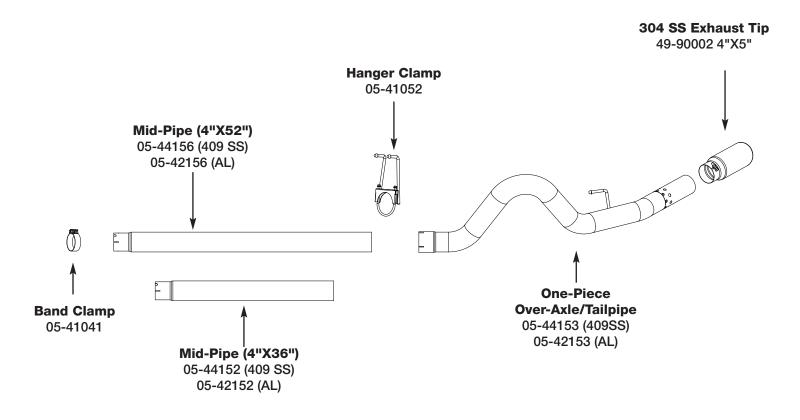
**Step 1:** (Read Instructions prior to installation) Remove your stock exhaust from the rear of your truck working your way forward. The spare tire and heatshield will need to be removed for exhaust replacement. Take caution not to damage the factory isolation mounts as they will be reused. It is recommended to not fully tighten the clamps until the entire system has been installed.
