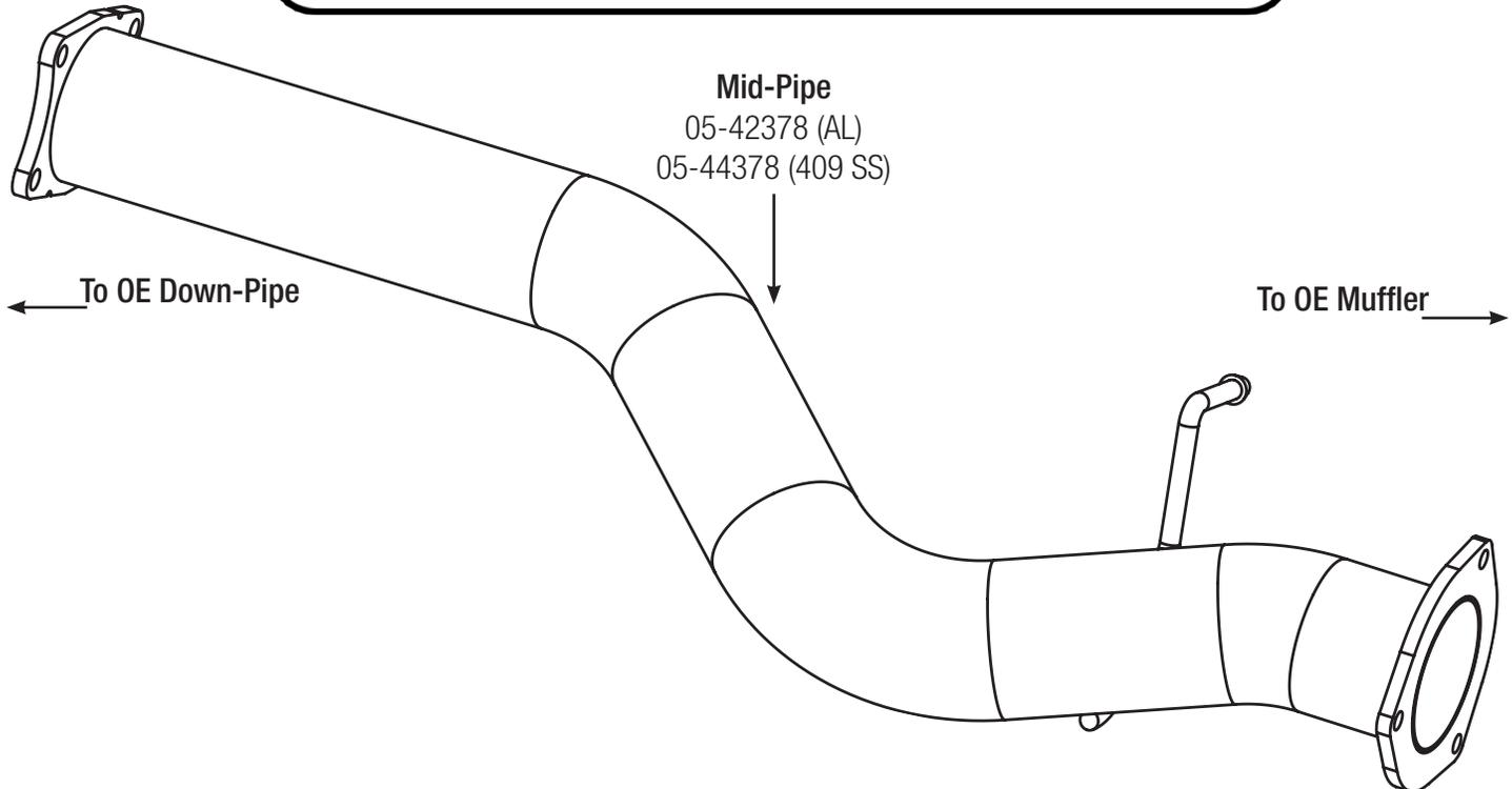
**Step 1: (Read Instructions prior to installation)** Disconnect sensors at the connections. Take caution as not to damage any sensors. Remove CAT/DPF section of your trucks exhaust working your way forward. Take caution not to damage the factory isolation mounts as they will be reused. **It is recommended to not fully tighten the clamps until the entire system has been installed.**
