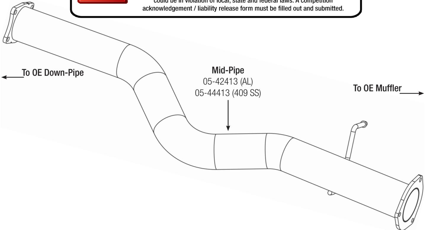
**Step 1: (Read Instructions prior to installation)** Disconnect sensors at the connections. Take caution as not to damage any sensors. Remove CAT/DPF section of your trucks exhaust working your way forward. Take caution not to damage the factory isolation mounts as they will be reused. **It is recommended to not fully tighten the clamps until the entire system has been installed.**
