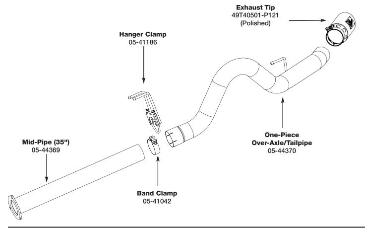
Step 1: (Read Instructions prior to installation) Remove your stock exhaust from the rear of your truck working your way forward. The spare tire and heat shield will need to be removed for exhaust replacement. Take caution not to damage the factory isolation mounts as they will be reused. It is recommended to not fully tighten the clamps until the entire system has been installed.
