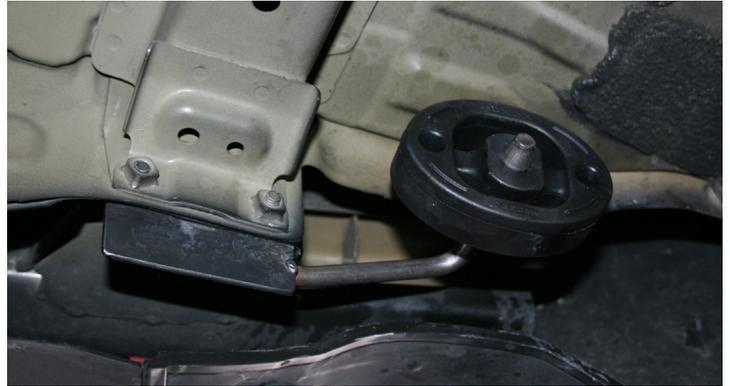
**Step 8:** Install the resonator pipe rubber hanger mount back onto the chassis and the original (x3) nuts removed from step 3 and tighten.
