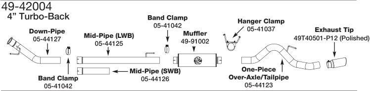
Step 1: (Read Instructions prior to installation) Remove your stock exhaust from the rear of your truck working your way forward. It may be necessary to cut the pipes if the slip joints are stuck. Take caution not to damage the factory isolation mounts as they will be reused. It is recommended to not fully tighten the clamps until the entire system has been installed.
