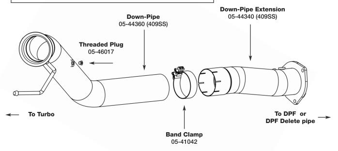
**Step 1:** (Read Instructions prior to installation) Disconnect sensors at the connections. Take caution as not to damage any sensors. Remove the CAT/DPF section of your trucks exhaust working your way forward. Take caution not to damage the factory isolation mounts as they will be reused. **It is recommended to not fully tighten the clamps until the entire system has been installed.**
