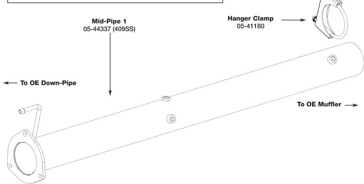
**Step 1:** (Read Instructions prior to installation) Disconnect sensors at the connections. Take caution as not to damage any sensors. Remove the CAT/DPF section of your trucks exhaust working your way forward. Take caution not to damage the factory isolation mounts as they will be reused. It is recommended to not fully tighten the clamps until the entire system has been installed.
