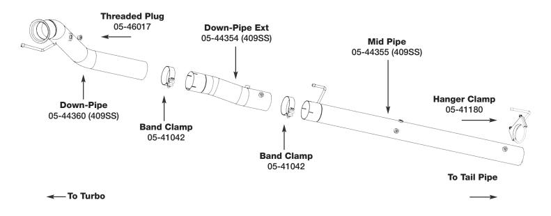
**Step 1:** (Read Instructions prior to installation) Disconnect sensors at the connections. Take caution not to damage any sensors. Remove the CAT section of your trucks exhaust working your way forward. Take caution not to damage the factory isolation mounts as they will be reused. It is recommended to not fully tighten the clamps until the entire system has been installed.
