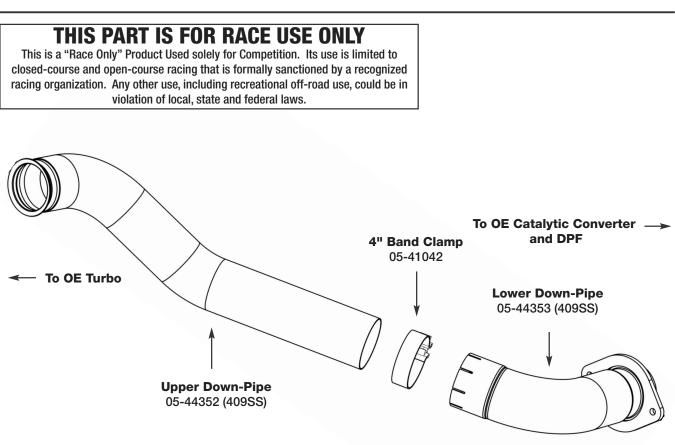
**Step 1: (Read Instructions prior to installation)** Remove your stock downpipe from the truck working your way forward. **It is recommended to not fully tighten the clamps until the entire system has been installed.**
