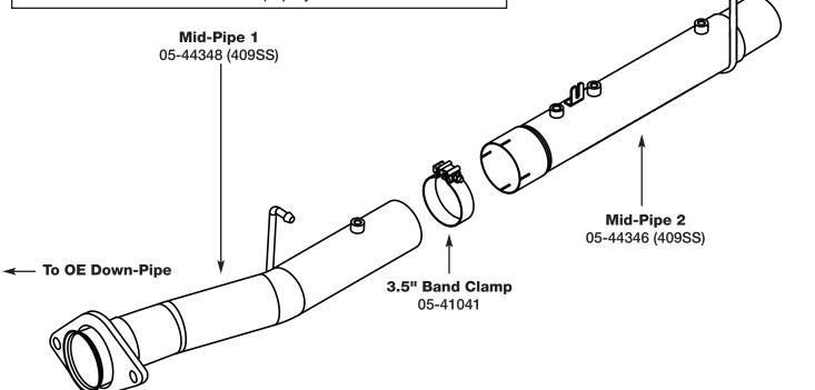
**Step 1:** (Read Instructions prior to installation) Disconnect sensors at the connections. Take caution as not to damage any sensors. Remove the CAT/DPF section of your trucks exhaust working your way forward. Take caution not to damage the factory isolation mounts as they will be reused. It is recommended to not fully tighten the clamps until the entire system has been installed.
