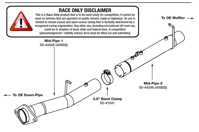
Step 1: (Read Instructions prior to installation) Disconnect sensors at the connections. Take caution as not to damage any sensors. Remove the CAT/DPF section of your trucks exhaust working your way forward. Take caution not to damage the factory isolation mounts as they will be reused. It is recommended to not fully tighten the clamps until the entire system has been installed.
