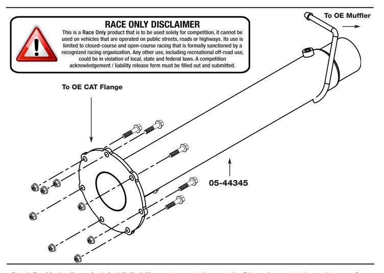
**Step 1:** (Read Instructions prior to installation) Disconnect sensor at the connection. Take caution as not to damage the sensor. Remove the DPF section of your trucks exhaust working your way forward. Take caution not to damage the factory isolation mounts as they will be reused. The original gasket can be reused or a new one will need to be sourced from your Ford dealer **It is recommended to not fully tighten the clamps until the entire system has been installed.**
