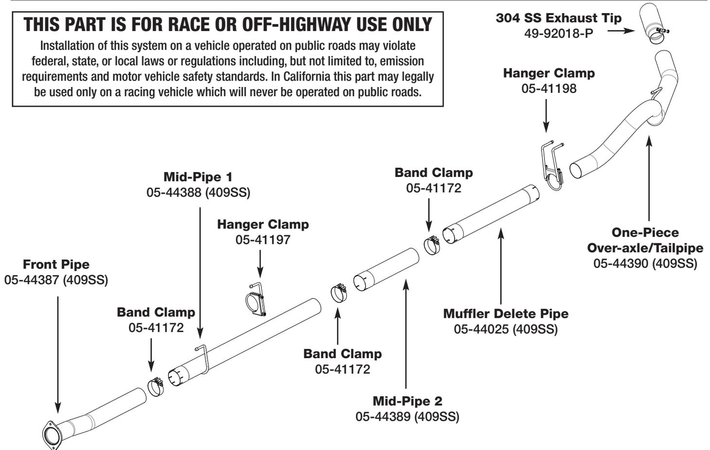
**Step 1: (Read Instructions prior to installation)** Remove your stock exhaust from the rear of your truck working your way forward. Take caution not to damage the factory isolation mounts as they will be reused. Disconnect sensors at the connections. Take caution as not to damage any sensors. **It is recommended to not fully tighten the clamps until the entire system has been installed.**
