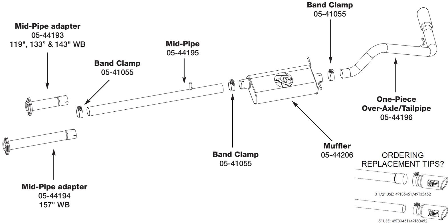
**Step 1: (Read Instructions prior to installation)** Remove your stock exhaust up to the catalytic converter from the rear of your truck working your way forward. Take caution not to damage the factory isolation mounts as they will be reused.
