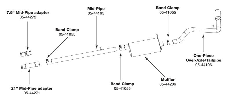
**Step 1:** (Read Instructions prior to installation) Remove your stock exhaust up to the catalytic converter from the rear of your truck working your way forward. Take caution not to damage the factory isolation mounts as they will be reused.
