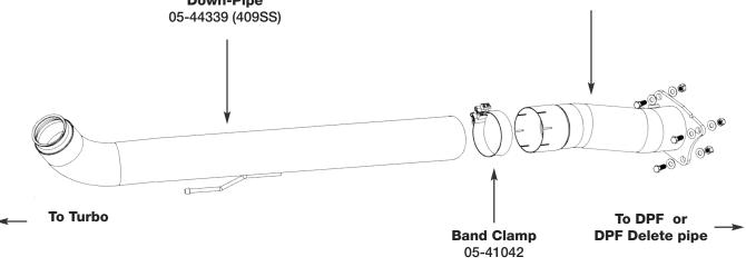
Step 1: (Read Instructions prior to installation) Disconnect sensors at the connections. Take caution as not to damage any sensors. Remove the CAT/DPF section of your trucks exhaust working your way forward. Take caution not to damage the factory isolation mounts as they will be reused. It is recommended to not fully tighten the clamps until the entire system has been installed.
