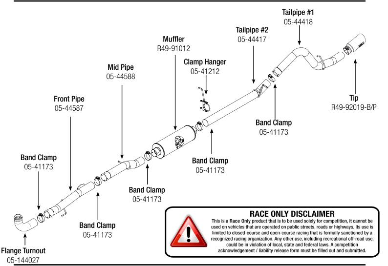
**Step 1: (Read Instructions prior to installation)** Remove the stock exhaust from the rear of the truck working your way forward. Take caution not to damage the factory isiolation mounts as they will be reused. Disconnect sensors at the connections. Take caution as not to damage any sensors. It is recommended to not fully tighten the clamps until the entire system has been installed.
