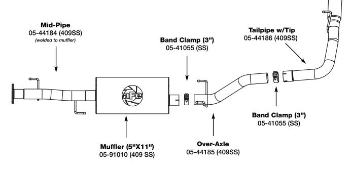
**Step 1:** (Read Instructions prior to installation) Remove your stock exhaust from the rear of your truck working your way forward. Take caution not to damage the factory isolation mounts as they will be reused. It may be helpfull to lubricate the isolation mounts prior to disassembly. *It is recommended to not fully tighten the clamps until the entire system has been installed.*
