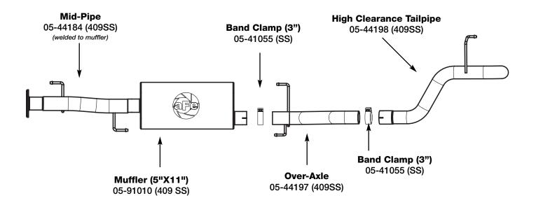
**Step 1:** (Read Instructions prior to installation) Remove your stock exhaust from the rear of your truck working your way forward. Take caution not to damage the factory isolation mounts as they will be reused. It may be helpfull to lubricate the isolation mounts prior to disassembly. It is recommended to not fully tighten the clamps until the entire system has been installed.
